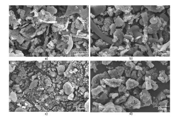
**Figure 2.** SEM micrographs of the powder obtained from a) Chondrilla nuculla (Alassio), b) Chondrilla nuculla (Porto Fino), C) Chondrosia reniformis and d) Thymosia sp.
