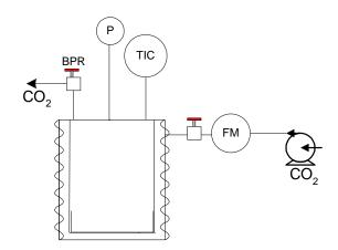
**Figure 1.** Schematic representation of extraction equipment for carbon dioxide acidified water. BPR – back pressure regulator, P – pressure transducer, TIC, temperature controller, FM, flow meter.
